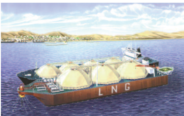
Artist impression of an LNG FSRU with a Hamworthy regasification plant
