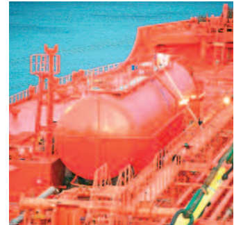
Heavy VOC components converted into pure liquid VOC fuel (an LPG mix of mainly propane and butane).
