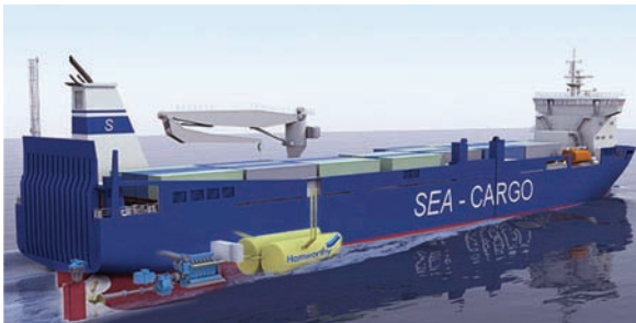
Complete gas propulsion system delivered by Hamworthy Gas Systems and Rolls-Royce Marine
