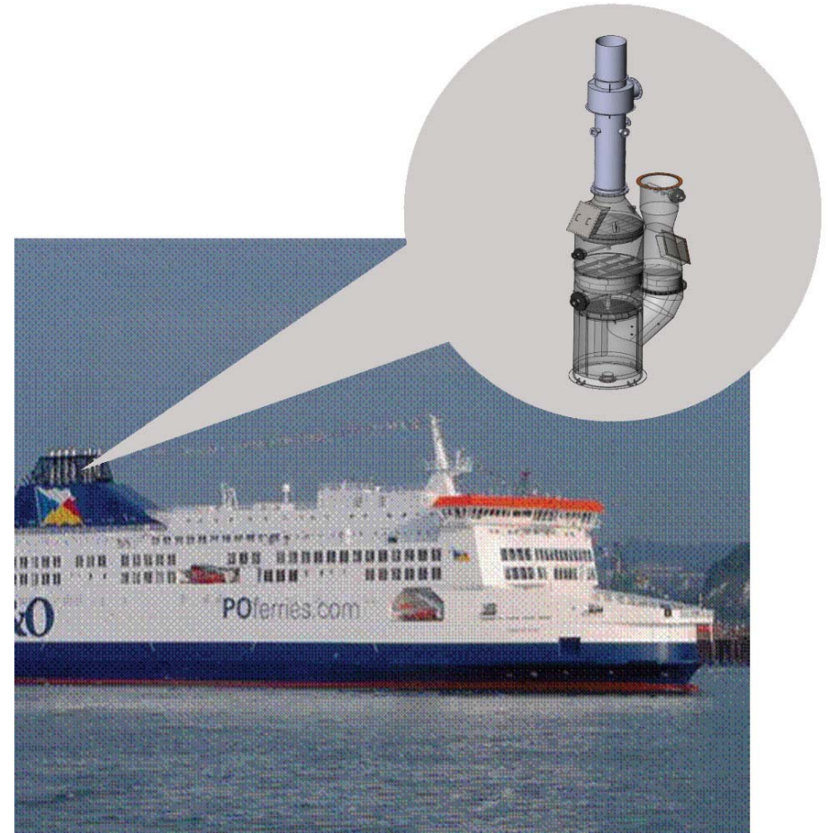
P&O Ferries Pride of Kent fitted with Hamworthy Krystallon's SOx abatement technology
